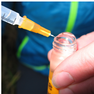
Figure 1: Adding \text{ZnCl}_2 to a MIMS sample. Half of my MIMS samples received the preservative before being stored.
